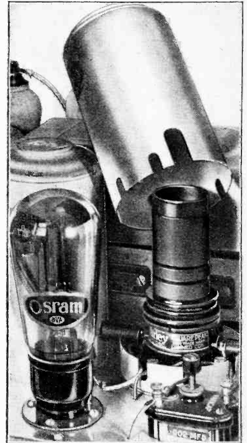
The oscillator coil of "The Wireless World" Monodial A.C. Superhet with screening cover removed.
