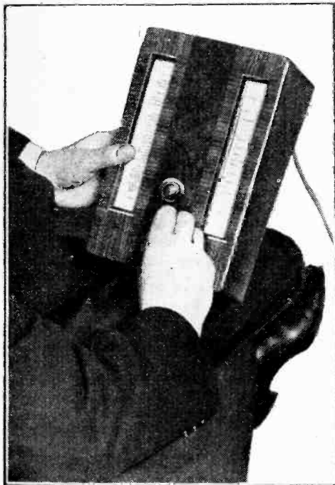
With the Telecontrol unit all the normal adjustments of the receiver can be made in comfort at the fireside.
