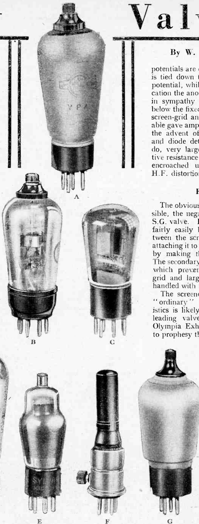
Typical new valves: (A) Mullard VP4, a variable-mu screened H.F. pentode; (B) Marconi double-diode triode, MHD4; (C) Mullard PM2B, twin Class "B" output valve; (D) Tungram PX46 single Class "B" valve, two of which will give 21 watts speech output; (E) Sylvania 6A7 Pentagrid; (F) Marconi Catkin pentode MPT4; (G) Tungram SE2018 variable-mu A.C.-D.C. valve.
