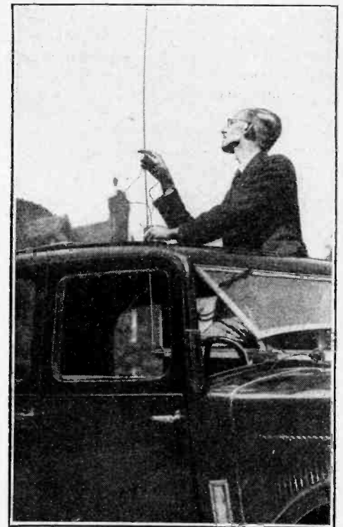
"ULTRA-SHORTS" RECEPTION ON A CAR. Mr. L. H. Thomas (GQB) demonstrating one method of reception on the very high frequencies. An ordinary aerial will be suitable for use with The Wireless World "Ultra Short Wave Two."
